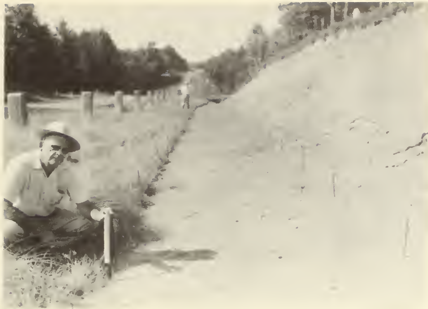
Figure 5.--Two rows of metal hub stakes spaced 6 by 6 feet are shown in the flow channel of a runoff plot. Annual measurements are made at 1-foot intervals around the squares of stakes and across the diagonals with equipment especially designed to determine the soil deposition or erosion that may have occurred in the flow channel.
